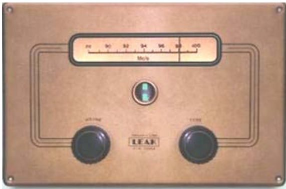
Above; an early Leak Trough-Line FM tuner with the pressed steel front, dating between 1955 and 1959.
